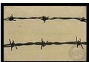
**BARBED WIRE (1873):** In settling the Great Plains, wooden fences were expensive and hard to acquire. Single-strand wire fencing was easily broken by cattle. The introduction of barbs locked into double-strand wire mass-produced by machinery and rolled on large spools solved both problems, but radically altered the nomadic life of Native Americans. Later it was used to protect military units in the time of war, to confine prisoners and mark territorial boundaries.
