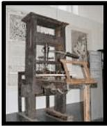
**PRINTING PRESS (1440):** In Germany, Johannes GUTENBERG invented a mechanical way of printing books by making a wooden press which used uniformly shaped pieces of metal, each with a different letter of the alphabet on its face, that could be endlessly rearranged to form new text. It gave the common man access to literature and encouraged record keeping that we, as genealogists, so deeply appreciate.
